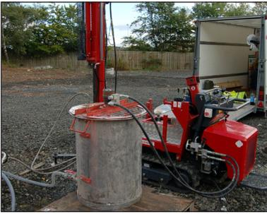
The compact nature of our rig allows us to access restricted areas through spaces as small as standard width doorways by dismounting the drive mast and operating remotely from the power source.
